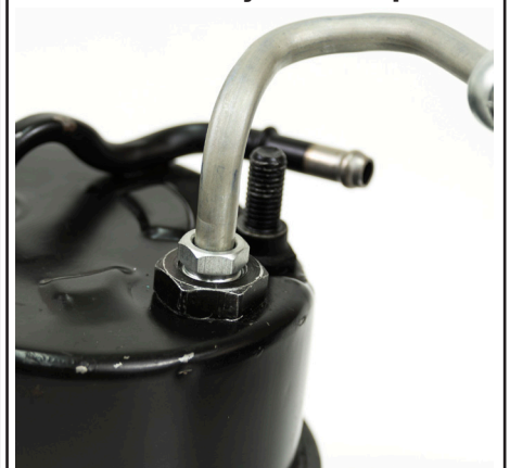
Fit Mackay Hose Directly To Pump
