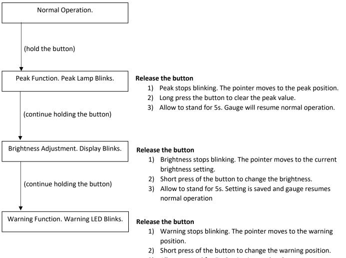
3) Allow to stand for 5s. Setting is saved and gauge resumes normal operation.
