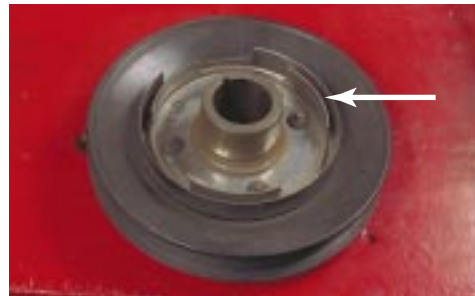
Figure 21-45 A crankshaft pulley for a six-cylinder engine has three interrupter rings.
