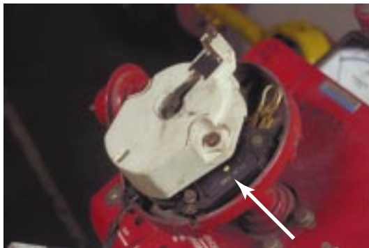
Figure 21-31 The control module mounted inside a GM HEI distributor.
