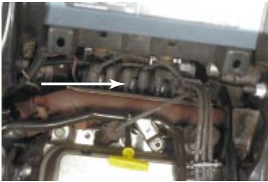
Figure 21-38 A coil pack for a distributorless ignition system.
