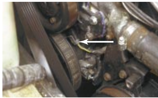
Figure 21-48 A camshaft position sensor mounted on the timing chain cover.
