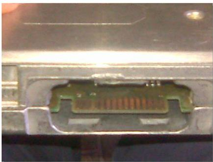
3. Once you have removed all of this lacquer, use some sandpaper (600 grade works well) to bring the terminals up to a shine. Finish it off by giving it a good clean with a rag and some methylated spirits as per the picture (left). **Note: Failure to follow these steps will lead to issues with the connection!**
